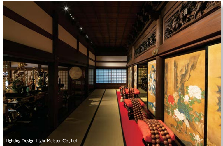
Micro Light Cannon fixtures with 3000K LEDs and a 24 degree lens illuminate this entire wall.
