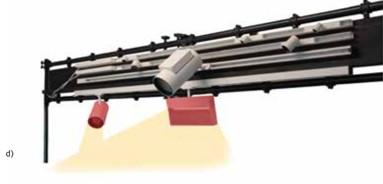
Settings of the luminaires on the support structure for the Sacra Conversazione: Configurations 1 (a), Configuration 2 (b), Configuration 3 (c) and Configuration 4 (d)
